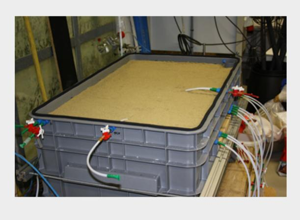
Box filled with soil and collector model
