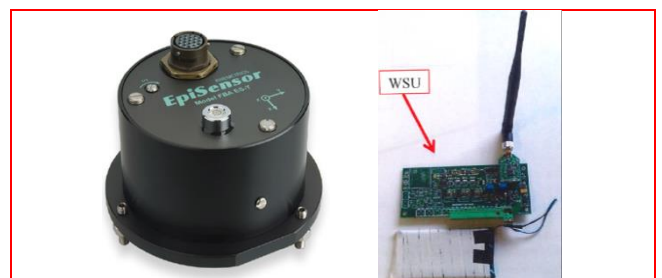
Fig. 3 Device equipment. WSU means wireless station unit.
