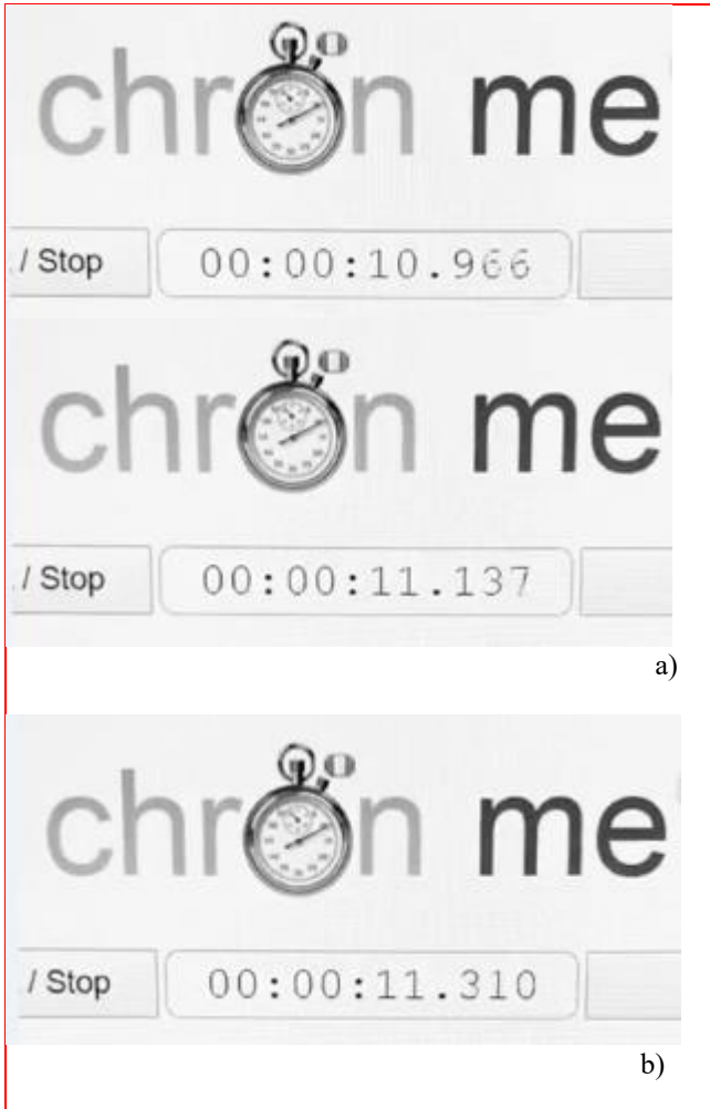
Fig. 6 Video progress for checking the actual frames per second rate: a) images 1 and 5; b) image 9.
