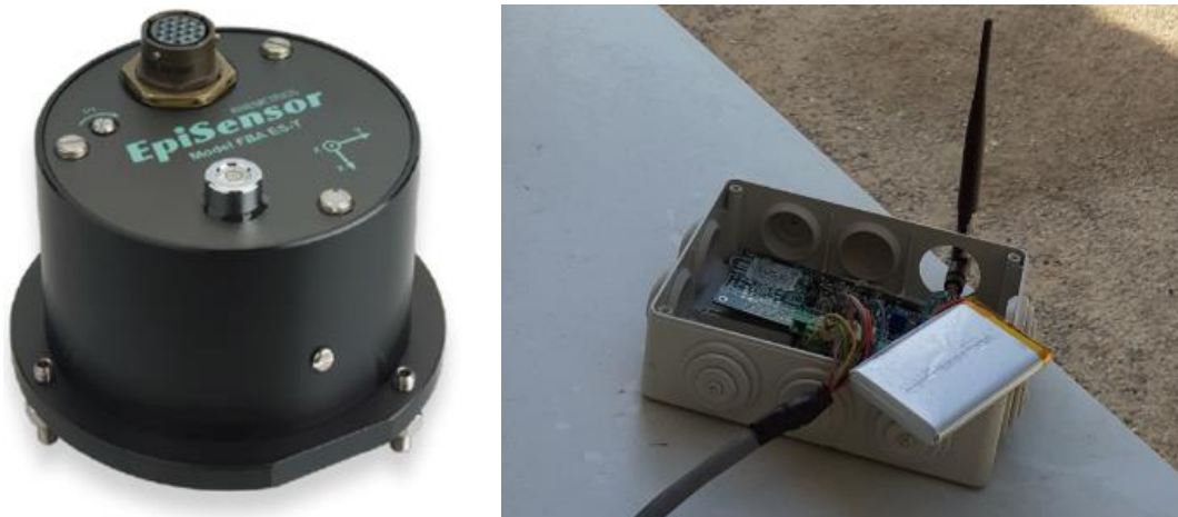
Figure 4: Device equipment. Left: EPISENSOR Model FBA ES-T accelerometers; Right: Wireless Data Acquisition, collection and transmission System (WDAS)
