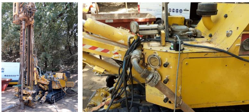
Fig. 6 Drilling machine (left); The accelerometer on the drilling machine (right)
